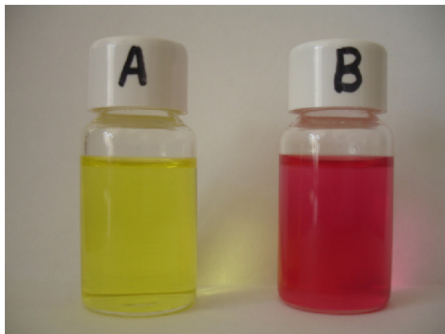
Fig. 9. The colour change of NI2TEA in DMF ( c = 10^{-5} \text{ mol l}^{-1} ) on addition of NaOH.
